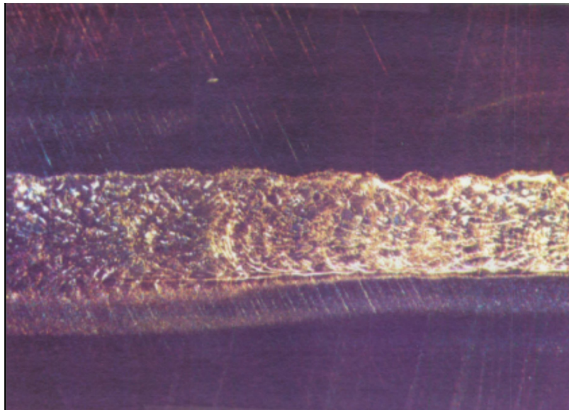
Figure 2. Weld ripples in stainless steel post-laser welding. 9
