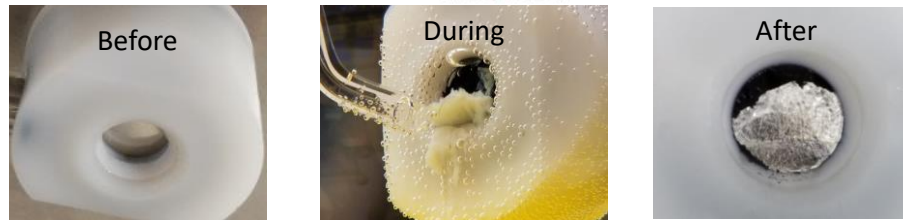
Figure 7. Polarization scans of Haynes 25 along with images showing the level of pitting from the test. (test results from Collins Aerospace).
