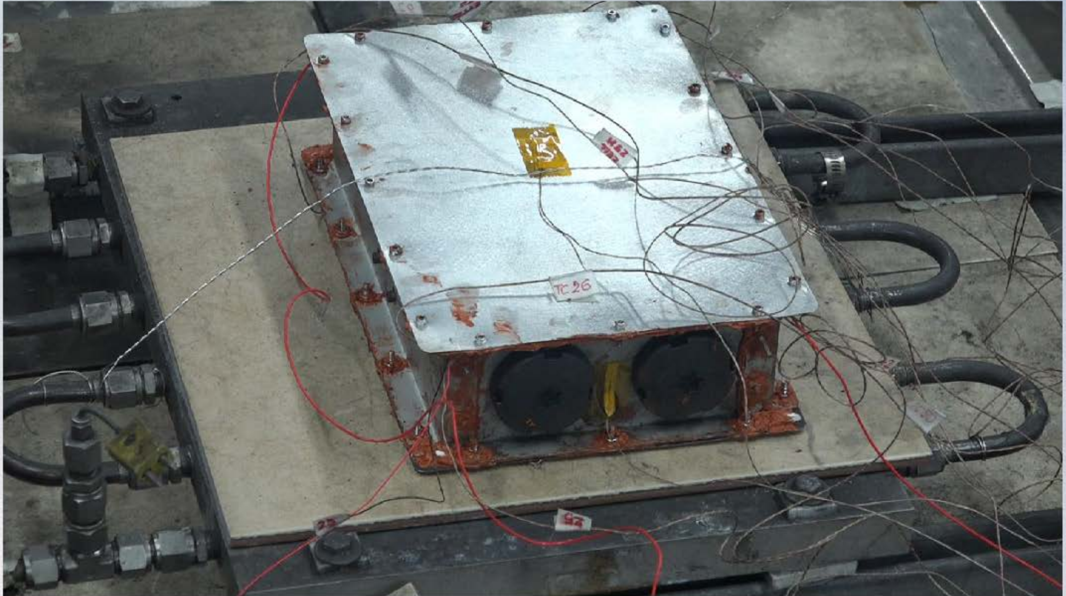
Zircar RS200 liner protecting the top and bottom Al panels
