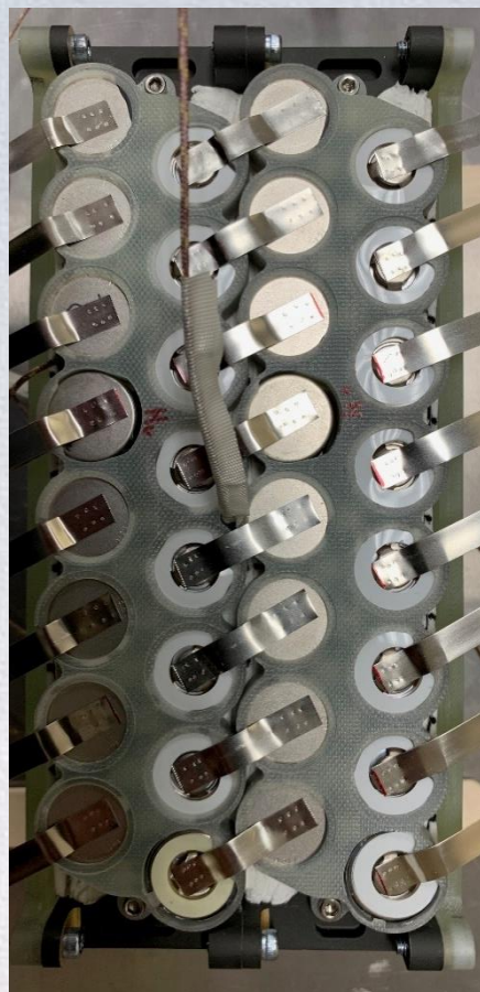
After welding cell interconnecting tabs
