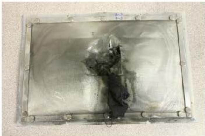
Post-test: Rivets intact, FR4 failed at some screw locations.
