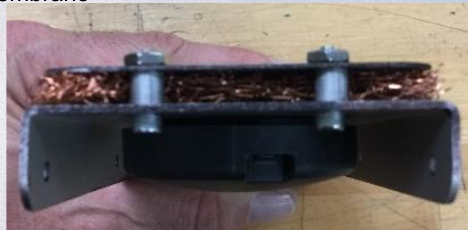
Double Gore vent panel using new flexible membrane
