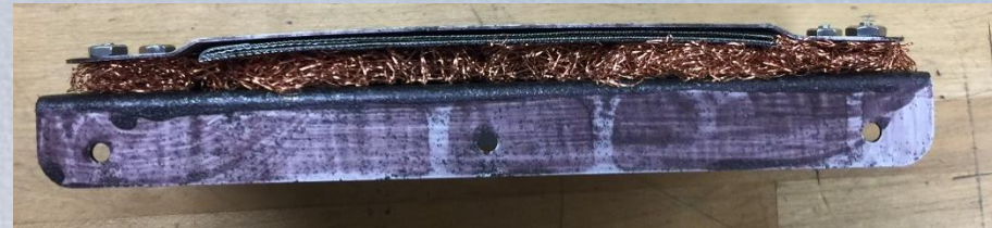
2 low pressure Gore vent ports backed by Steel screens, Cu mesh, and Al baffles
