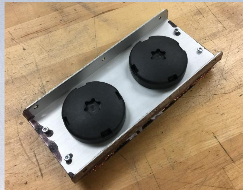
Double Gore vent panel using new flexible membrane
