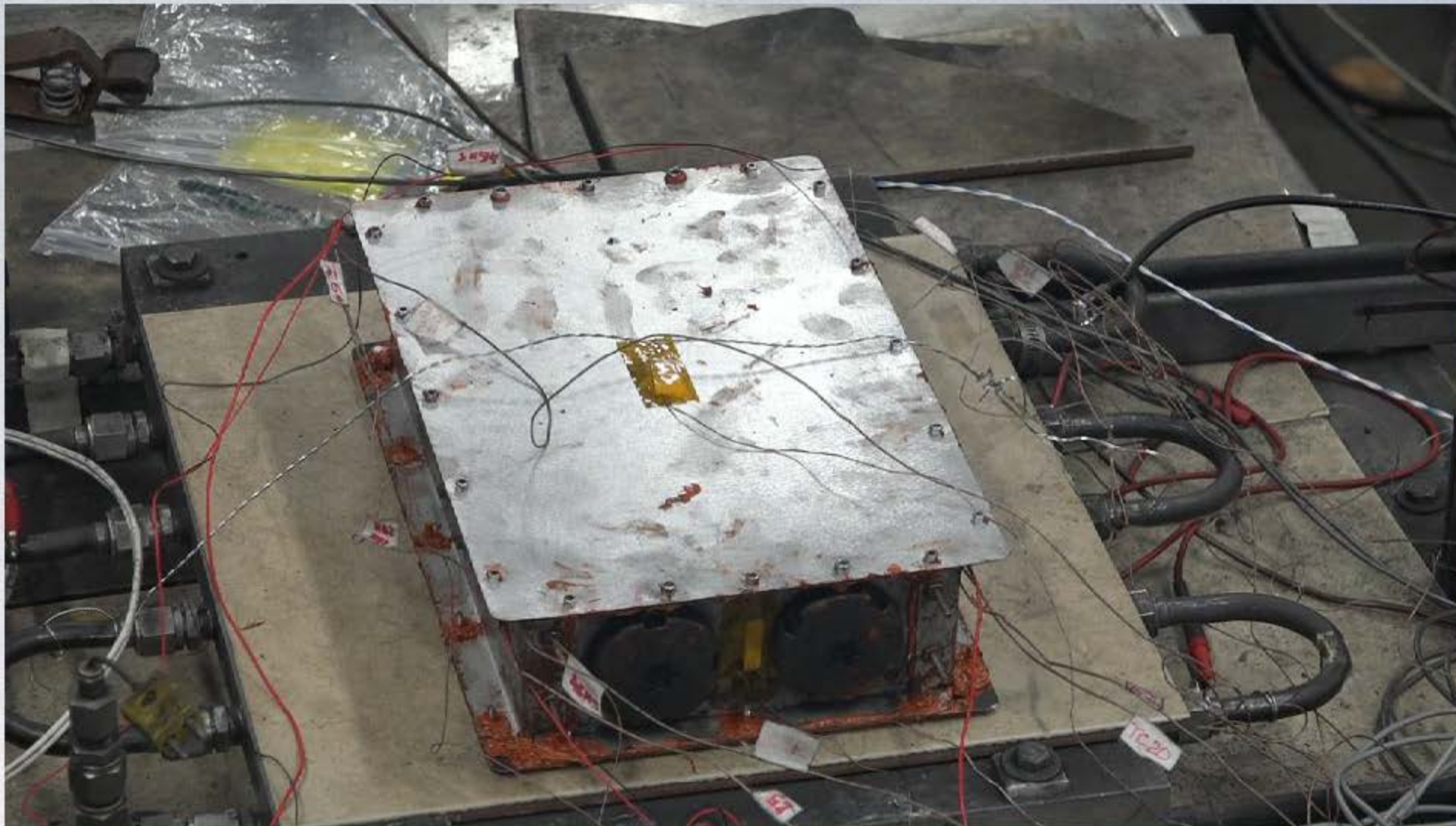
Kaowool material on top and bottom panels
