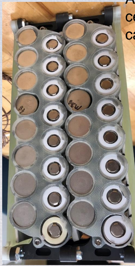
Ceramic putty cured in place
