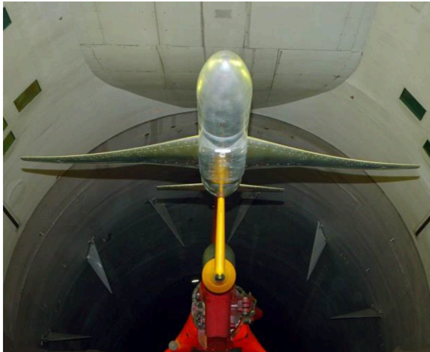
Fig. 32. The ONERA Large Reference Model installed in the ONERA S1MA wind tunnel.
