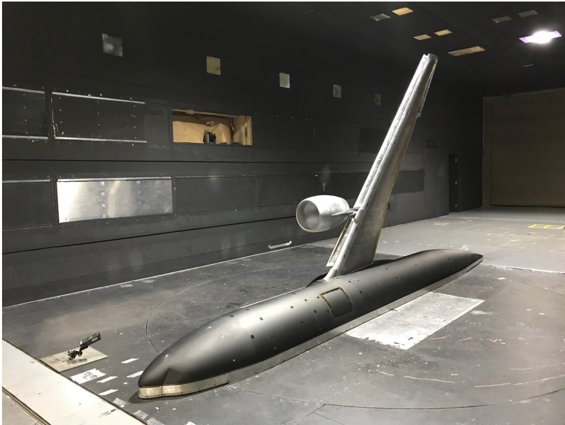
Fig. 34. Photo of the CRM-HL model installed in the 14- by 22-Foot Subsonic Wind Tunnel at the NASA Langley Research Center.
