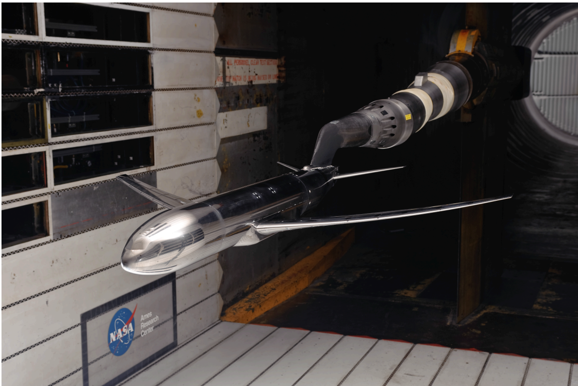
Fig. 5. Photo of the NASA Common Research Model in the Ames 11-Foot Transonic Wind Tunnel Facility.
