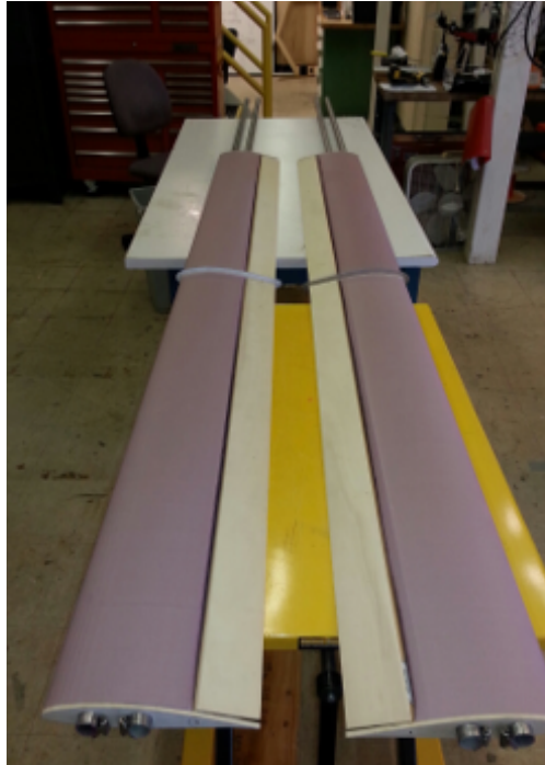
Fig. 25 Wings fabricated for wind tunnel testing of the docking mechanism. Note that each of the 10 ft span wings have inboard and outboard actuated ailerons used to selectively unload the wings during testing.
