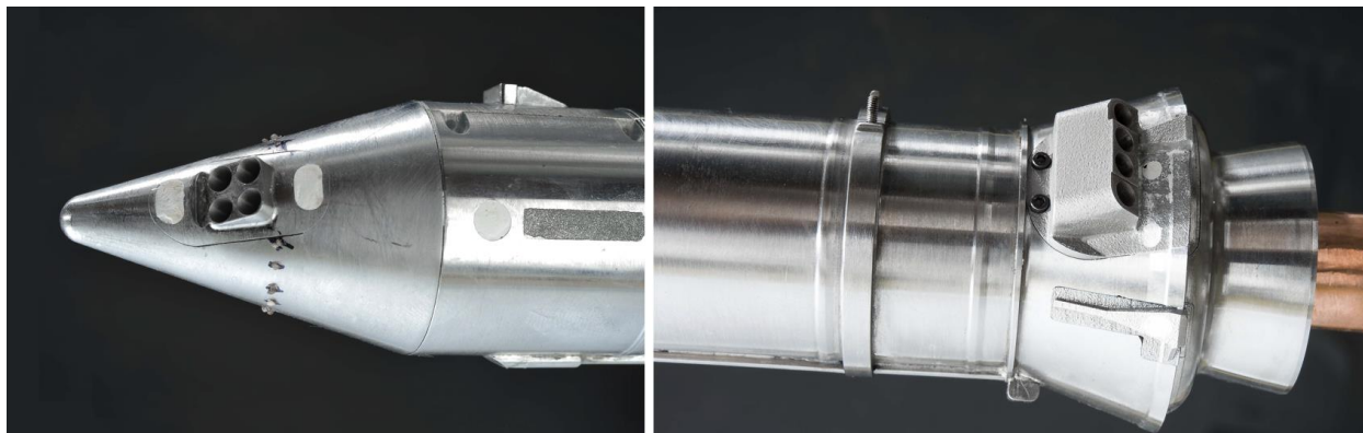
Figure 2. Detailed images of the SRB's forward (left) and aft (right) BSMs, oriented to show the left-hand BSMs studied in the current paper. Modified from Ref. 7 with permission of the authors.
