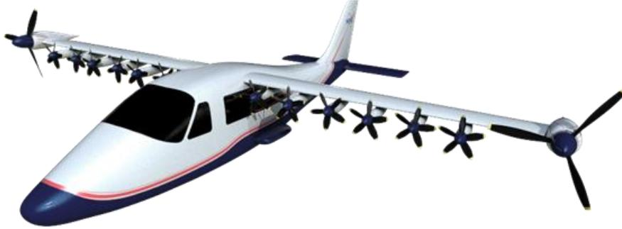
**Figure 1. SCEPTOR or X-57 electric motor powered aircraft.**
