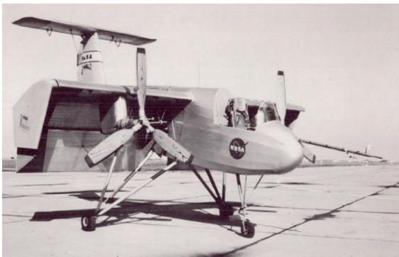
(a) Ryan VZ-3 deflected slipstream V/STOL aircraft, shown with slaps fully extended and with full-span leading edge slat installed [18].
