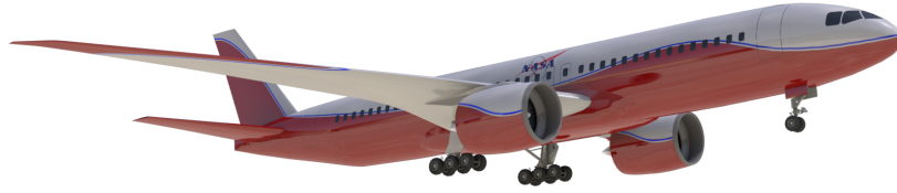
Fig. 1 An illustration of the conventional tube-and-wing architecture TW301M with engines under the wing is shown.
