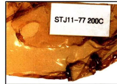
KSC Developmental Polyimide STJ 11-77 .02mm) - colored transparent self sealing
