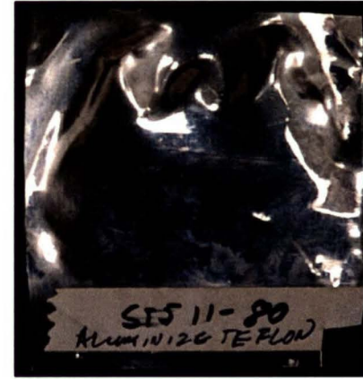
Aluminized Teflon (.063mm) with polyimide layer
