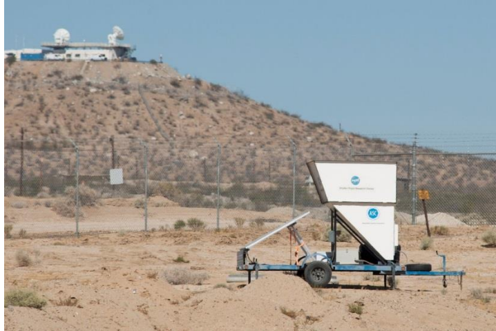
Figure 43. SODAR Model 4000 deployed at primary array for AFRC test.
