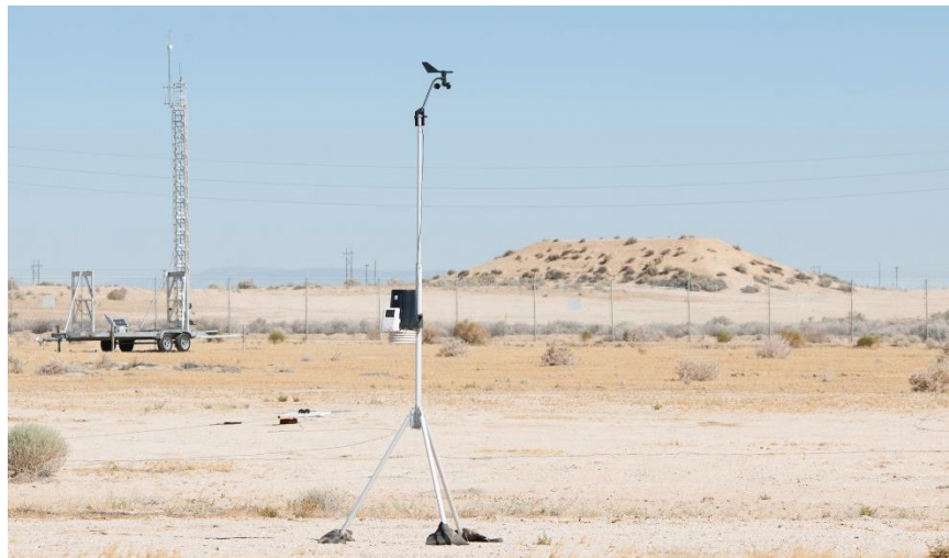
Figure 40. Weather station (in the foreground) deployed at the primary array. Ultrasonic anemometer on 10 m tower shown in background.
