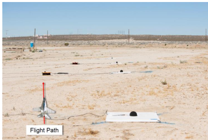
Figure 35. Microphones on ground boards at primary array.
