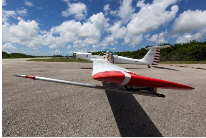
Figure 64. TG-14 motorized glider with microphone mounted under and forward of wingtip.
