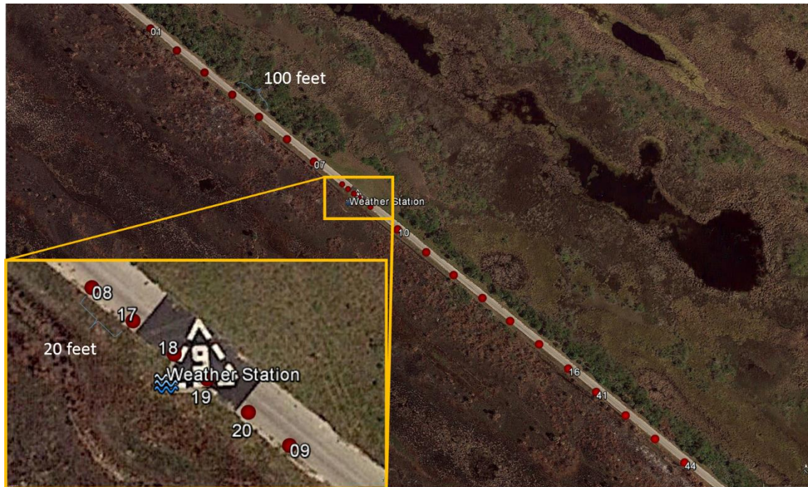
Figure 67. Secondary array layout showing microphone positions and weather station. Inset shows a zoom of the center of the array with finer spaced positions added for first week of measurements.
