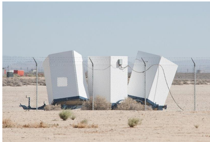
Figure 42. SODAR Model 2000 deployed at the primary array for the AFRC test.
