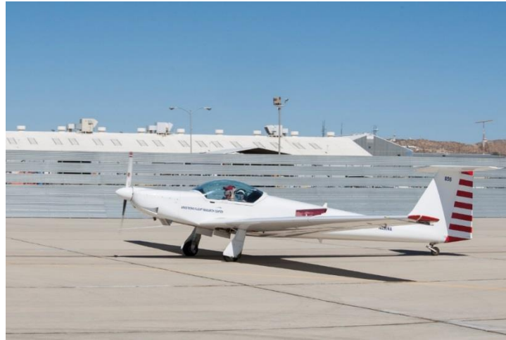
Figure 34. TG-14 motorized glider with microphone mounted under wingtip.
