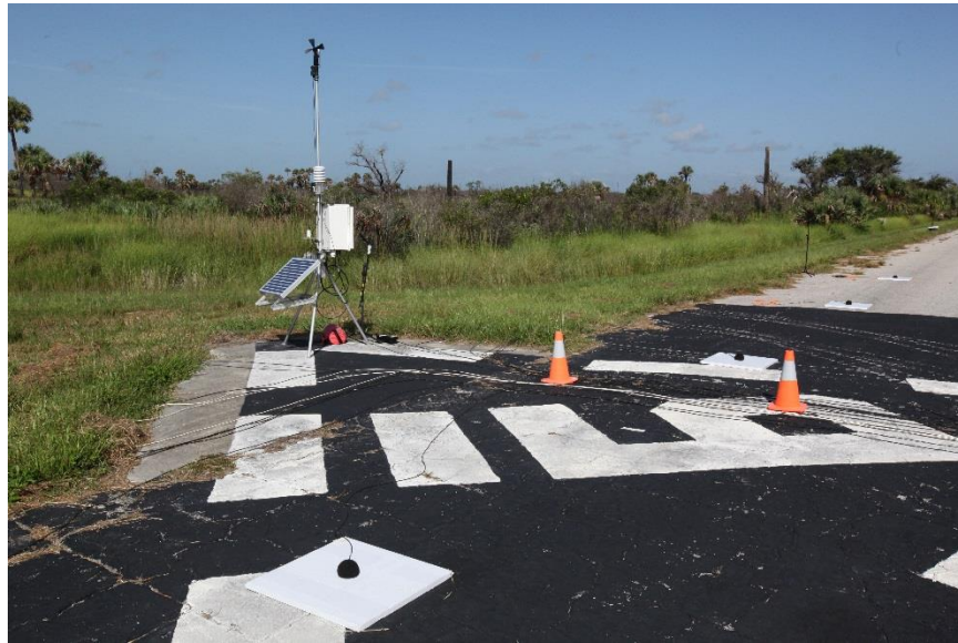
Figure 69. Weather station deployed at the secondary array.
