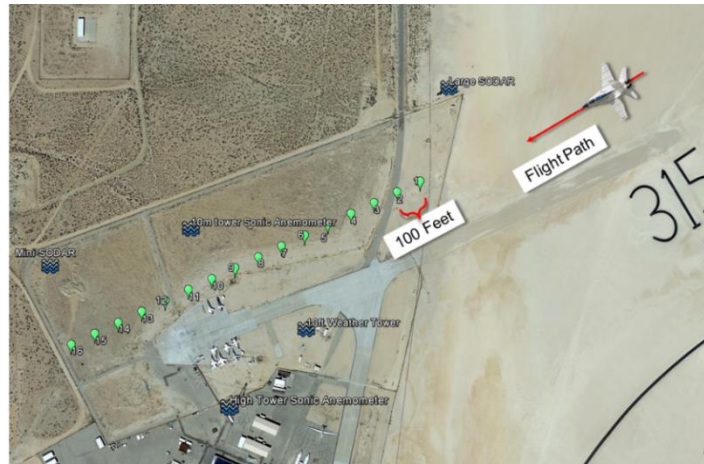
Figure 36. Primary array layout of microphones 1 through 16 and meteorological instrumentation.
