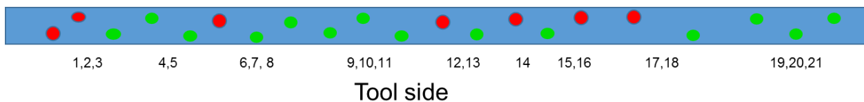
Figure 4: Schematic of the typical layout and numbering of the rods used to create wrinkling in the flat plate standards. The diameter of the rods shown in red are 0.1875 in. (0.476 cm) and the ones shown in green are 0.125 in. (0.3175 cm). Rod locations alternated between the third and fourth plies and between the 13 th and 14 th plies.
