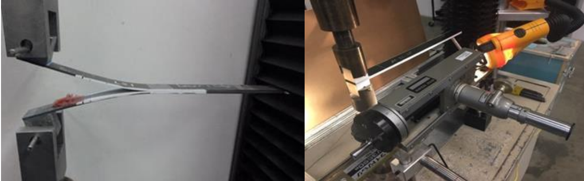
Figure 3. Double cantilever beam testing
