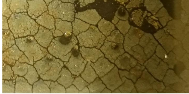
Figure 1. Condensed Molecular Contaminant Film (NASA/Elaine Seasly)
