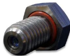
Figure 5. Image of the resin pressure sensor.
