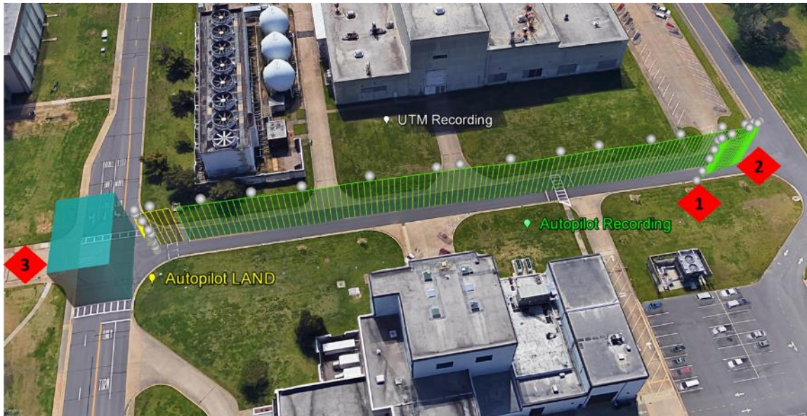
Figure 2. Example of a flight ending with an auto-land contingency maneuver to avoid geo-fence violation at street intersection. This flight included UTM tracking (Flight date 2017_07_20). Waypoints are shown as red diamonds. Vehicle positions as reported by the autopilot are shown as green and yellow lines extending from the vehicle altitude to ground. Vehicle positions as retrieved from the UTM tracking server are shown as grey spheres. The stay-out region is shown as the cyan box at middle left. Upon approaching the geofence (green position series), the Safeguard avionics detected an imminent geofence violation and initiated a landing (yellow position series). © Satellite map data: Google.
