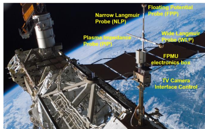
Fig. 2. The Floating Potential Measurement Unit (FPMU) showing the location of the WLP, NLP, FPP, and PIP as well as the electronics box and TVCIC (NASA image).
