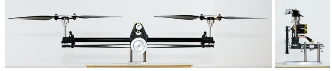
Figure 1. Dual rotor assembly from the front and side.
