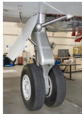
b) Fairings installed
