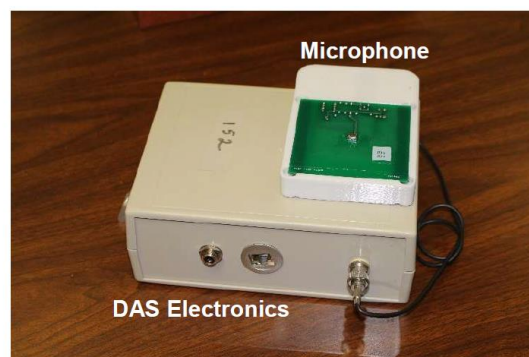
Figure 6. Microphone mounted on top of NeAR module.
