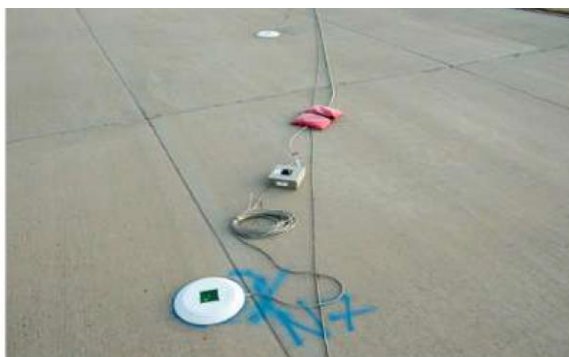
Figure 5. NeAR module installation at Edwards. The microphone is on the round plate. The NeAR module is the square box.
