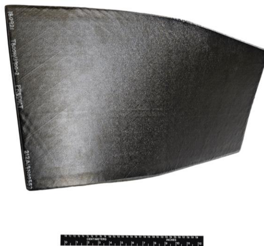
Figure 12. Cured and trimmed MDU.
