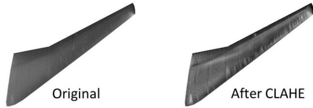
Fig. 7. Contrast enhancement of the heating layer image in Fig. 6 using CLAHE
