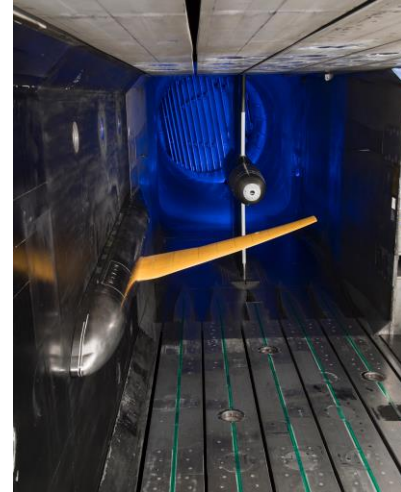
Fig. 1. CRM-NLF wing mounted in the NTF.
