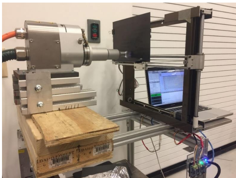
Figure 1 Atmospheric pressure plasma jet treatment system
