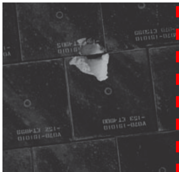
Damge to Shuttle Orbiter tiles
