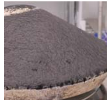
Ablated TPS on Stardust heat shield
