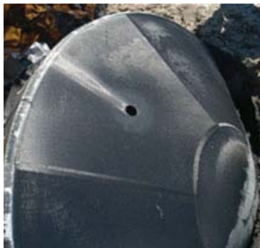
Attachment point cavities on Genesis heat shield
