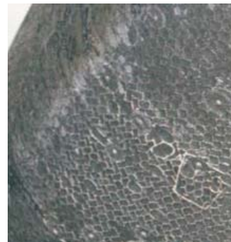
Ablated TPS on Apollo heat shield
