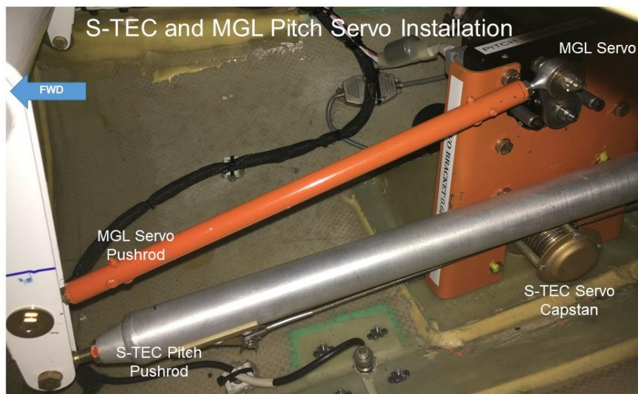
Figure 6. MGL Pitch Servo Installation.
