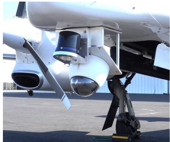
Figure 2: LiDAR and Point-Tilt-Zoom Camera Installed on Centaur
