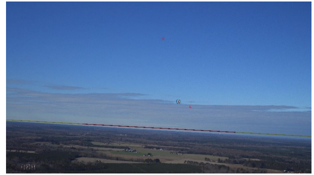
Fig. 17. Sample detector result where green is the difference detector and red is the morphological detector.
