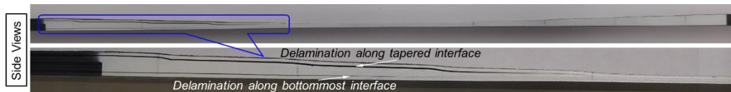
Figure 8. Post-test photographs of the fatigue tested specimen at NIAR showing the location and extent of delamination growth.
