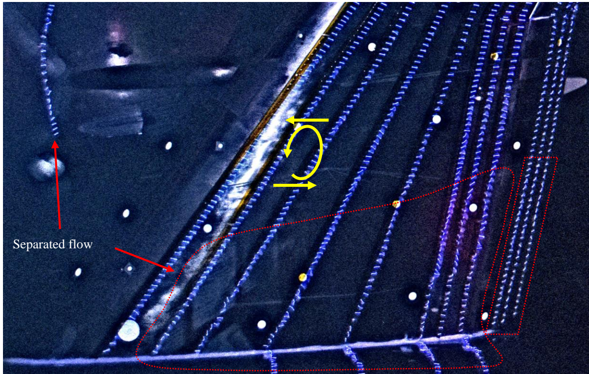
Fig. 30 Surface tuft flow visualization of the chine case at \alpha = 18^\circ .
