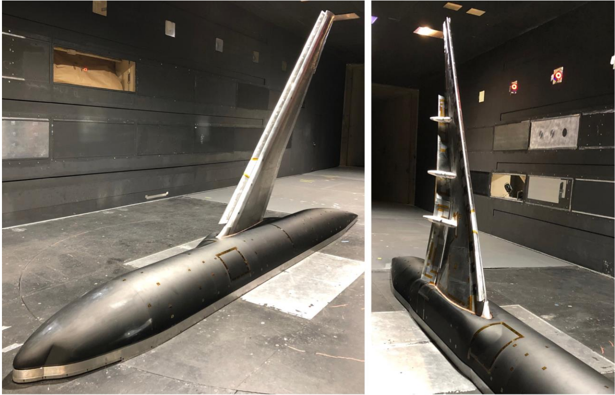
a) b) Fig. 13 The CRM-HL model in the 14x22 without the nacelle/pylon: a) upper surface, b) lower surface.
