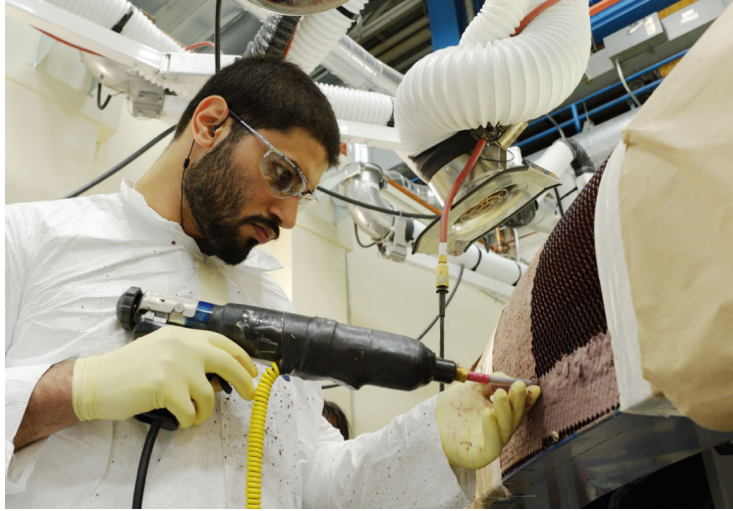
Figure 11. Manual injection process implemented on Orion EFT-1 heat shield ( https://www.nasa.gov/content/partnerships-make-missions-possible )
