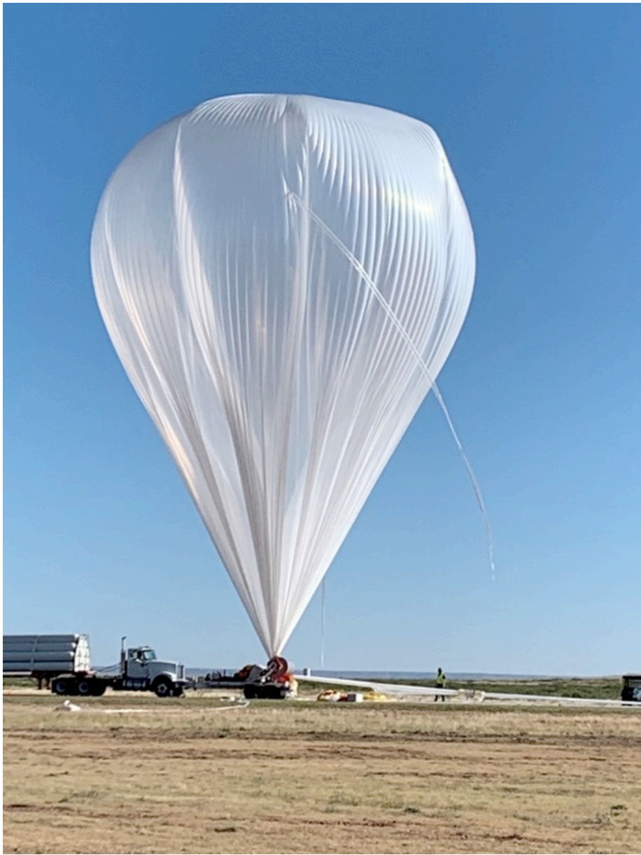
A balloon measuring over 1.1 million cubic meters carried BITSE to an altitude of 40 km.
