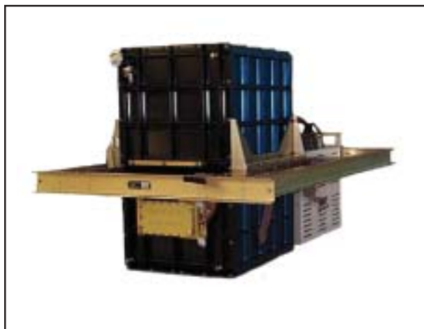
Figure 4-6. Photo of the CPL in flight configuration. The optical bench, shown in Figure 4-5, resides inside the blue box (top) to keep the optics clean, dry, and thermally stable. The entire package slides into the ER-2 wing pod.
