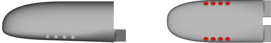
Fig. 1 Mid-L/D engine configuration evaluated for aerodynamic interference effects.
