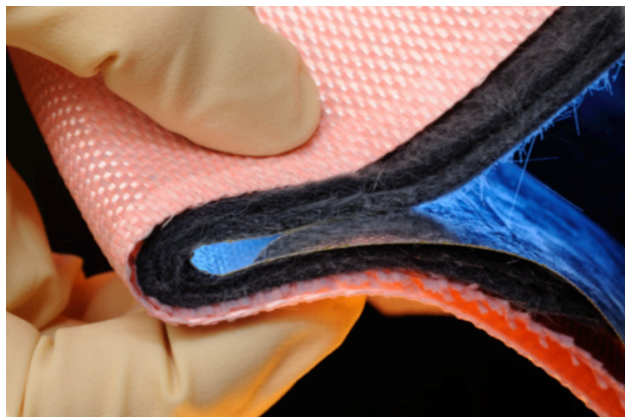
Fig. 5 Photo of first generation HIAD TPS
