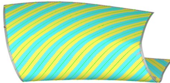
Figure 6. Example of tow paths on a complex contour tool.
