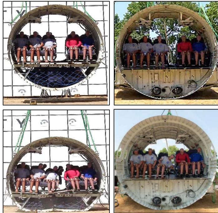
Figure 1. Pre- (upper) and Post- (lower) Test Photographs of Fokker F28 Component Tests: Forward Section (left) & Wingbox Section (right)
