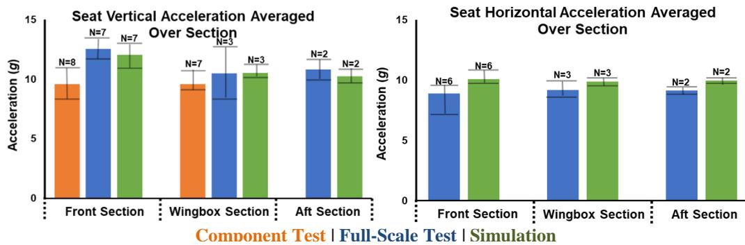
Figure 11. Comparison of Seat Accelerations Averaged over Section between Component Test, Full-Scale Test, and FEM Simulation
