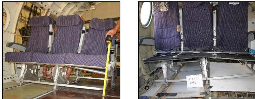
Figure 13. Seat Deformation in Component (left) and Full-scale Test (Right)
