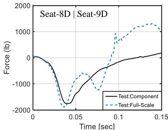
Figure 15. Comparison of Lumbar Load Response between Wingbox Section Component and Full-Scale Test
