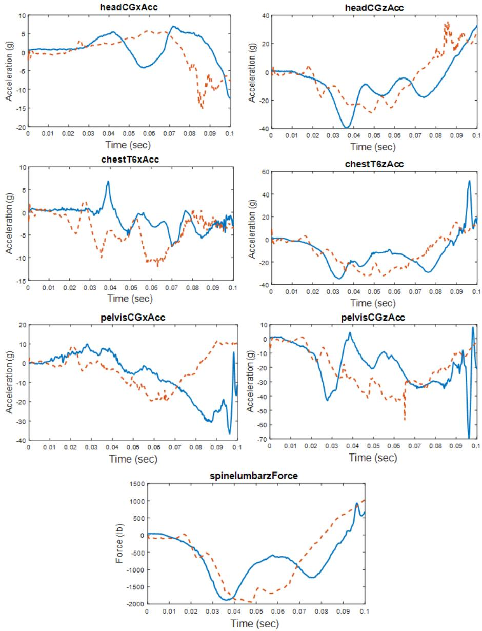
Figure 40. Seat 9D - Hybrid II Primary Impact Correlation Results (Simulated with FAA Hybrid III FEM)
