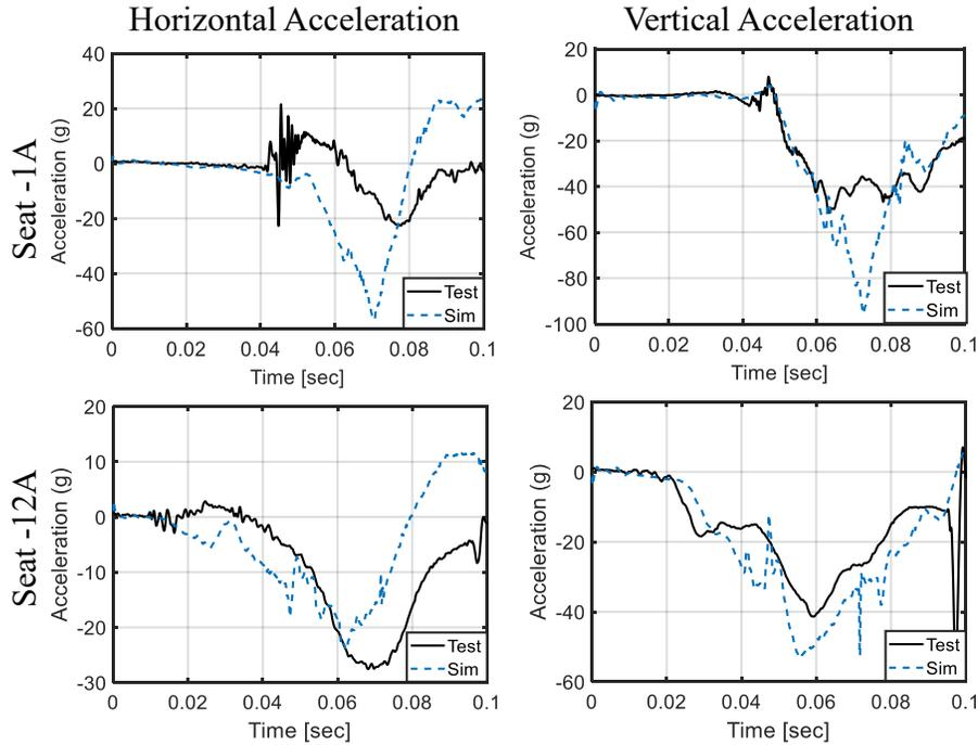
**Figure 24. Comparison of Pelvis Acceleration Predictions across Length of Aircraft**
