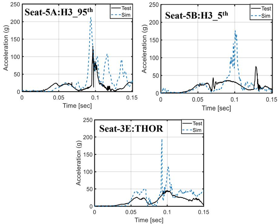
**Figure 27. Comparisons of Hybrid III -95<sup>th</sup>, -5<sup>th</sup>, and THOR Head Resultant Acceleration Response through Secondary Impact**
