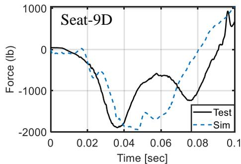
**Figure 21. Comparisons of Lumbar Load Response across Wingbox Section of the Full-Scale Aircraft**
