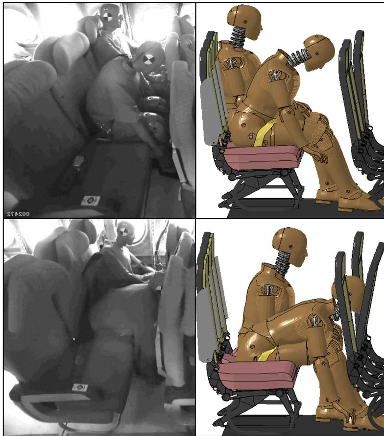
**Figure 23. . Kinematic Response Comparisons of Braced ATD between Test and Simulation: Initial Position (Top) and Peak Neck Extension (Bottom) – Seat 6B**
