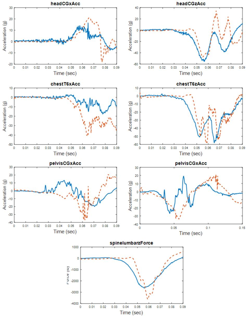
Figure 33. Seat 3D - Hybrid II Primary Impact Correlation Results (Simulated with FAA Hybrid III FEM)
