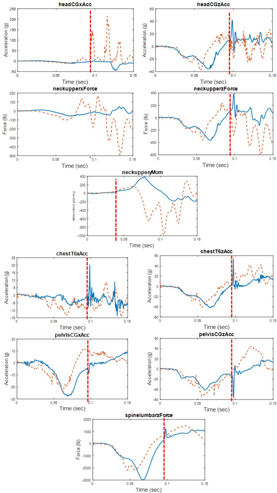
Figure 42. Seat 12A – FAA Hybrid III Primary & Secondary Impact Correlation Result
