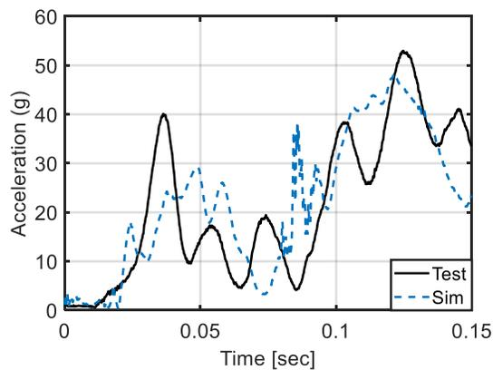
**Figure 29. Comparison of Head Resultant Acceleration Response through Secondary Loading without Seatback Contact – Seat 9D**
