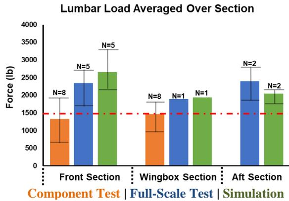
Figure 16. Comparison of Peak Lumbar Load Predicted by FEM Simulation and Measured in Component and Full-Scale Test
