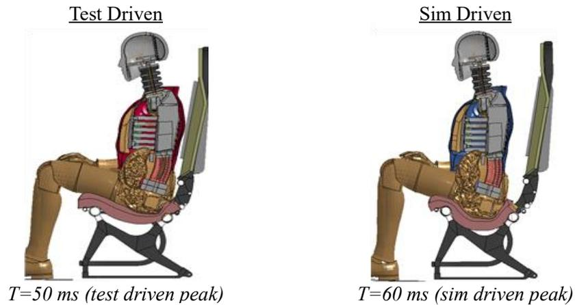
Figure 19. Kinematic Response Differences at Peak Lumbar Loading between Test and Simulation Driven Acceleration Conditions – Seat 3D
