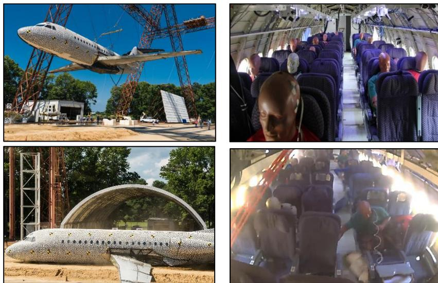
Figure 3. Pre- (upper) and Post- (lower) Test Photographs of Fokker F28-Full Scale Tests: External/Airframe (left) & Internal/ATDs (right)
