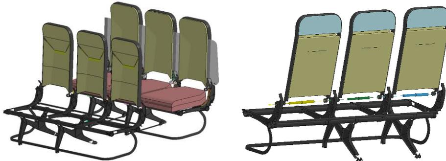
Figure 6. Seat Breakout FEM
