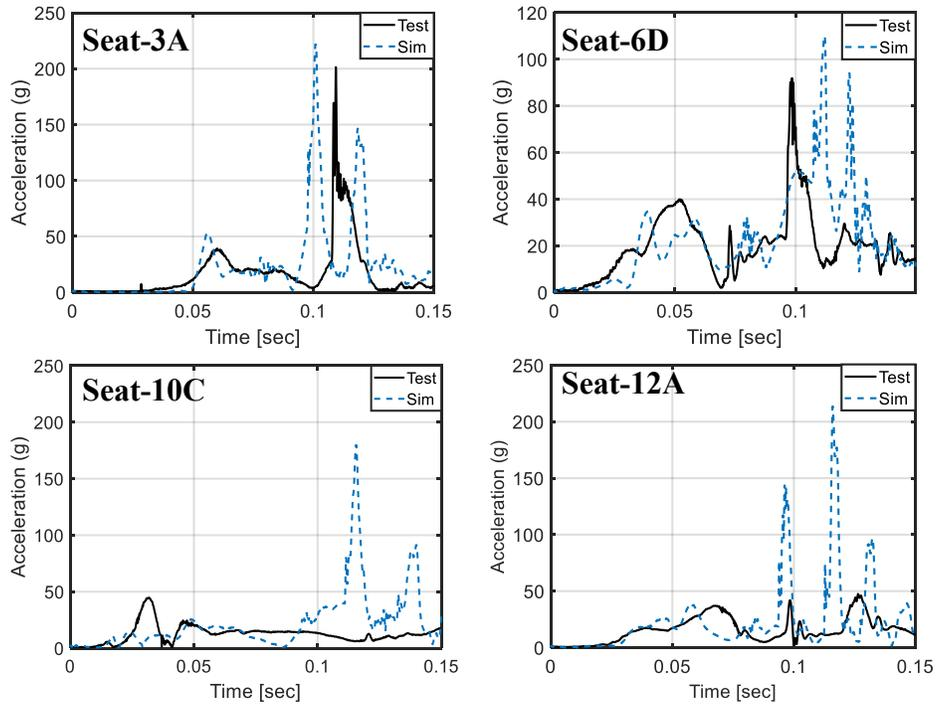
**Figure 26. Comparisons of FAA Hybrid III Head Resultant Acceleration Response through Secondary Impact**
