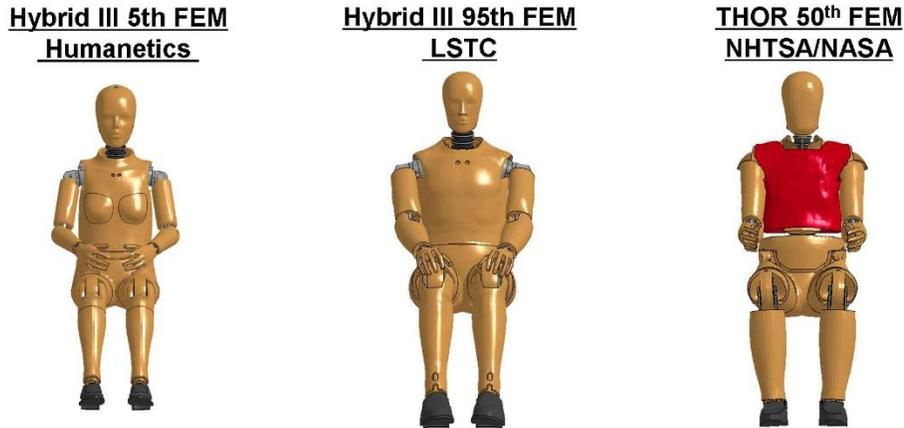
Figure 8. Hybrid III - 5<sup>th</sup>, -95<sup>th</sup>, and THOR FEMs
