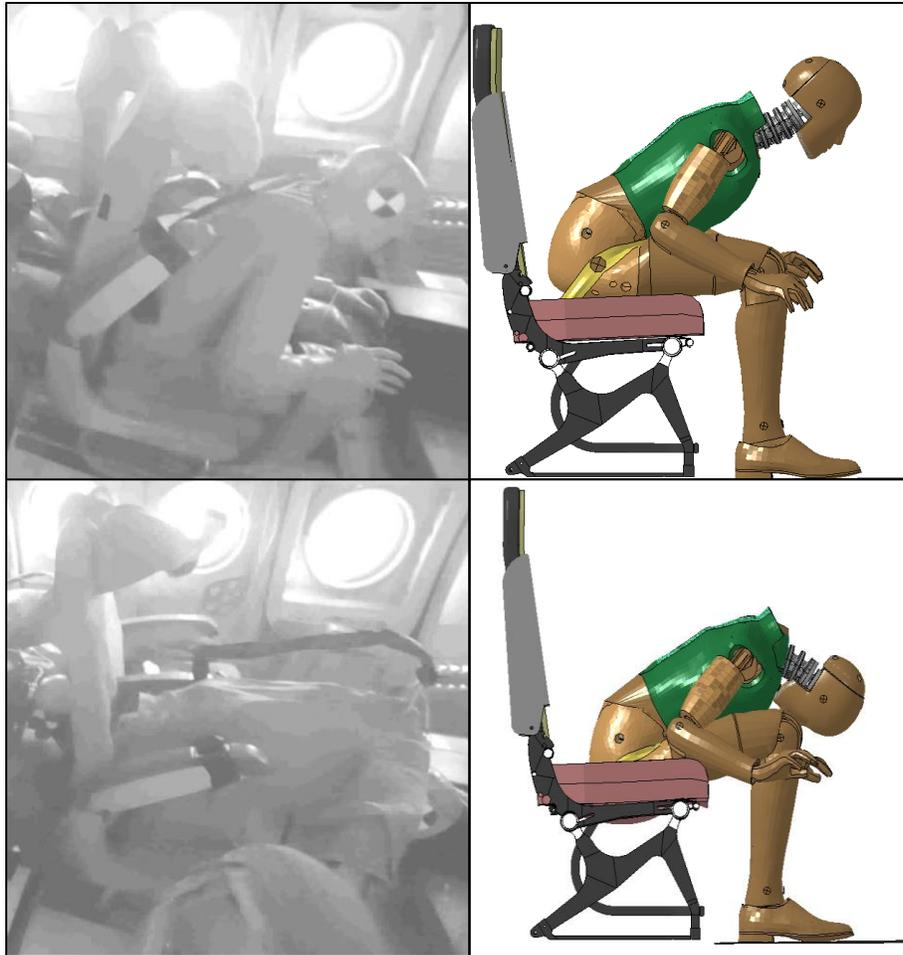
Figure 30. Kinematic Response Comparisons between Test and Simulation – Seat 9D
