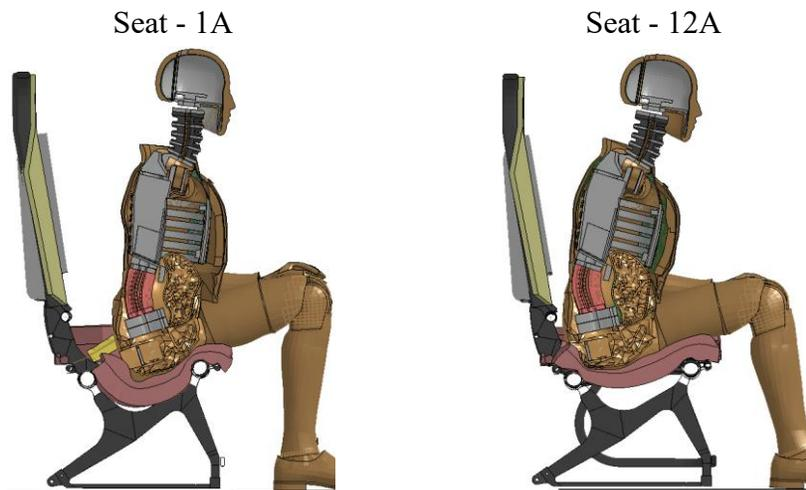
**Figure 25. Kinematic Response Comparison between Seat 1A and Seat 12A at Simulated Peak Pelvis Acceleration**
