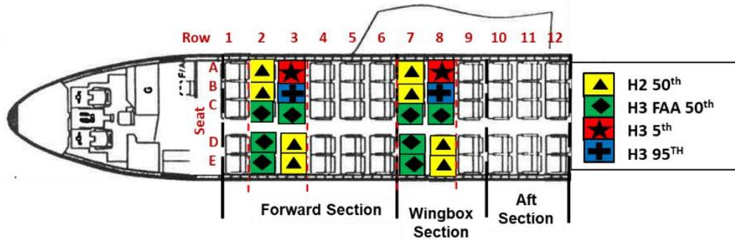
Figure 2. ATD Layout of Fokker F28 Component Tests
