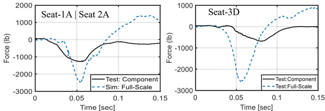
Figure 14. Comparison of Lumbar Load Response between Forward Section Component and Full-Scale Test
