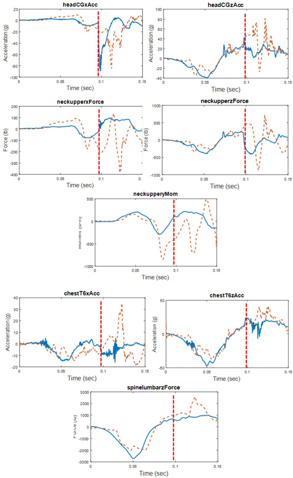
Figure 39. Seat 6D – FAA Hybrid III Primary & Secondary Impact Correlation Results
