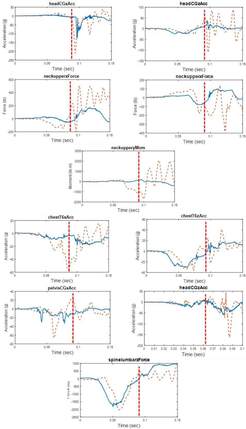
Figure 35. Seat 5A – Hybrid III 95<sup>th</sup> Primary & Secondary Impact Correlation Results
