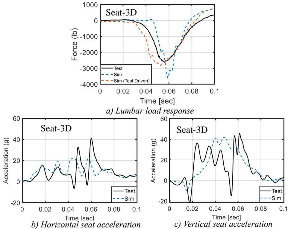
Figure 18. Lumbar Load Response Comparison between Test and Simulation Driven Acceleration Conditions – seat 3D
