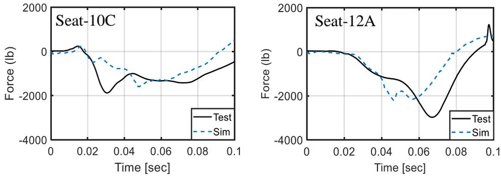
Figure 22. Comparisons of Lumbar Load Response across Aft Section of the Full-Scale Aircraft
