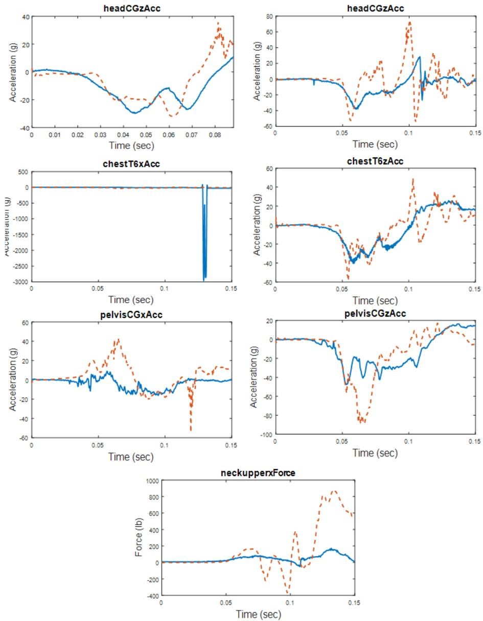
**Figure 31. Seat 1A - Hybrid II Primary Impact Correlation Results (Simulated with FAA Hybrid III FEM)**
