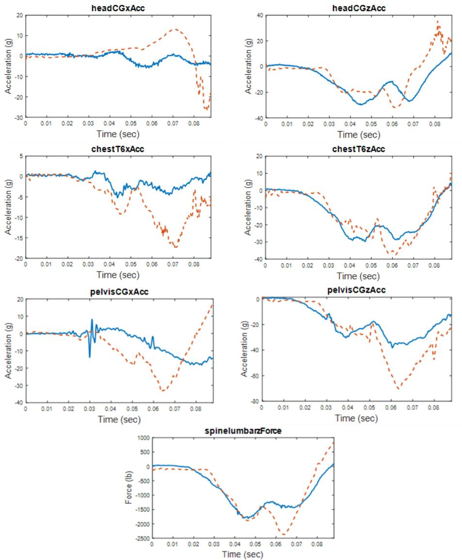
Figure 38. Seat 6B - Braced Hybrid II Primary Impact Correlation Results (Simulated with FAA Hybrid III FEM)
