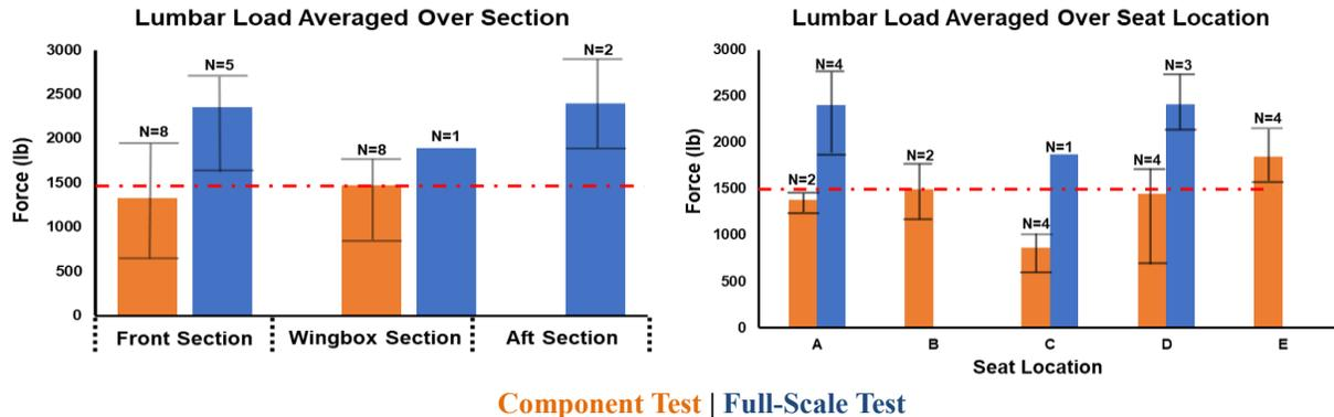
Figure 12. Comparison of Peak Lumbar Load Measured in Component and Full-Scale Test
