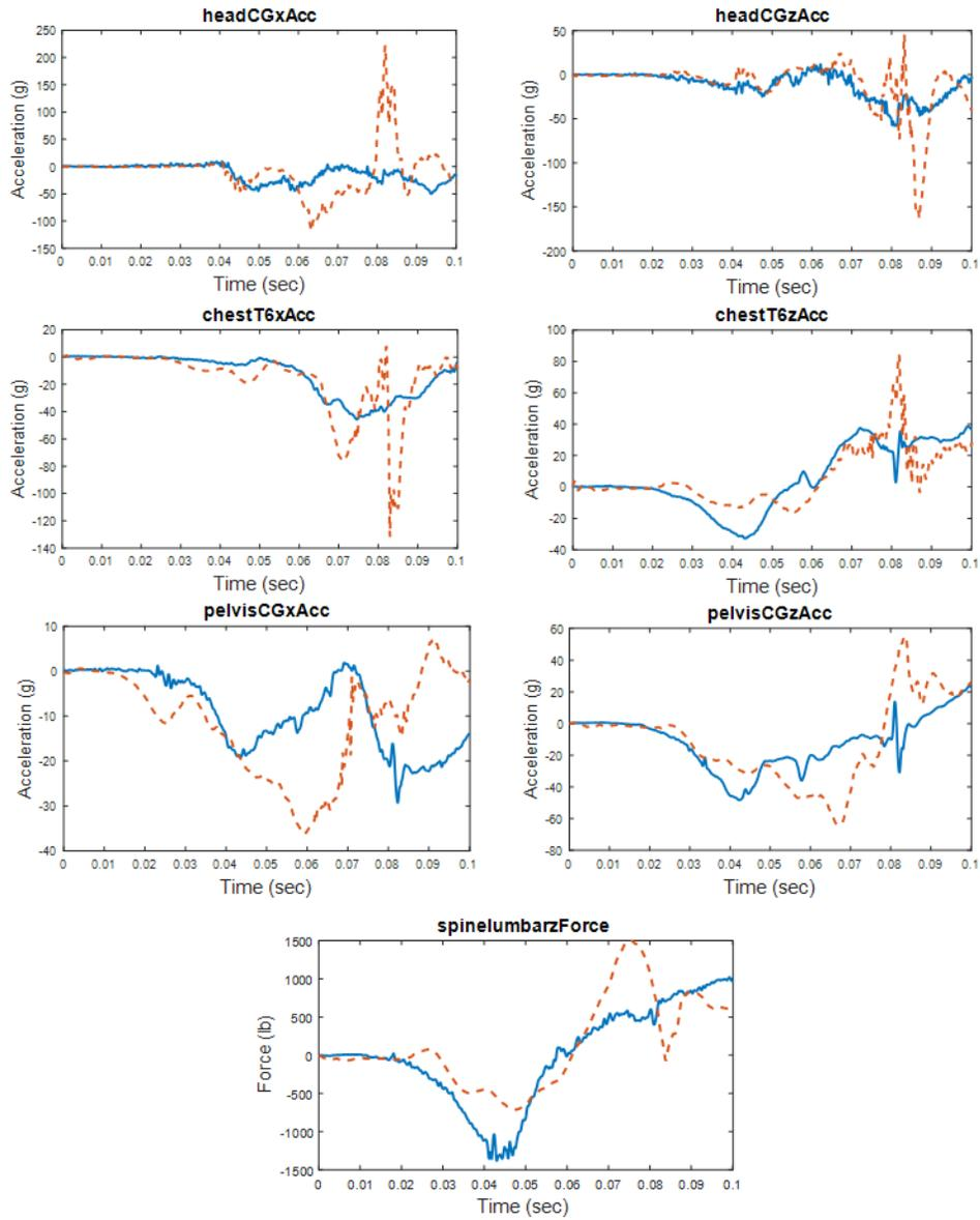
Figure 37. Seat 6A - Hybrid II Primary Impact Correlation Results (Simulated with FAA Hybrid III FEM)
