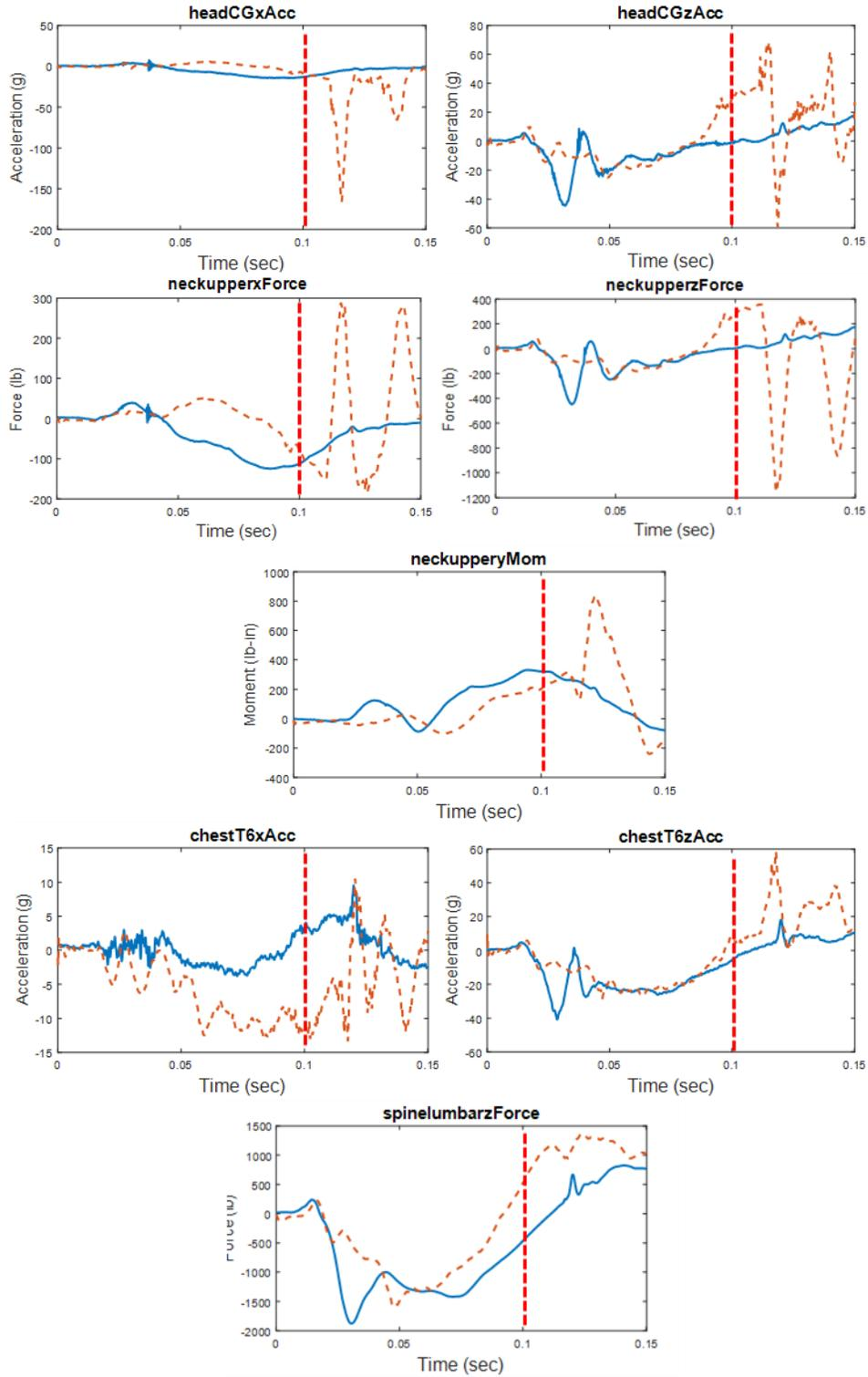
Figure 41. Seat 10C – FAA Hybrid III Primary & Secondary Impact Correlation Results
