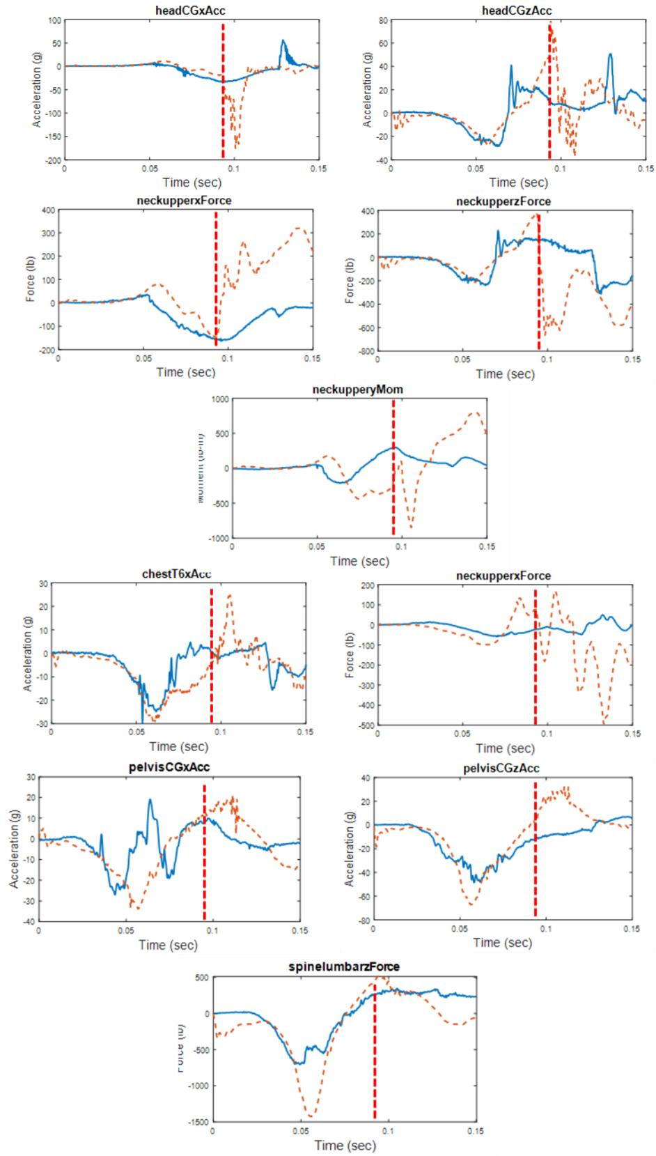
Figure 36. Seat 5B- – Hybrid III 5<sup>th</sup> Primary & Secondary Impact Correlation Results
