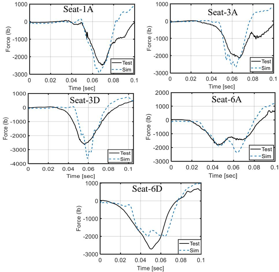
**Figure 17. Comparisons of Lumbar Load Response across Forward Section of the Full-Scale Aircraft**
