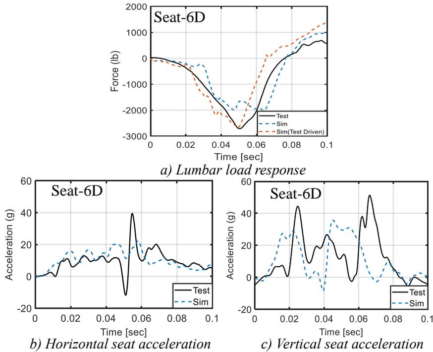
**Figure 20. Lumbar load Response Comparison between Test and Simulation Driven Acceleration Conditions – Seat 6D**
