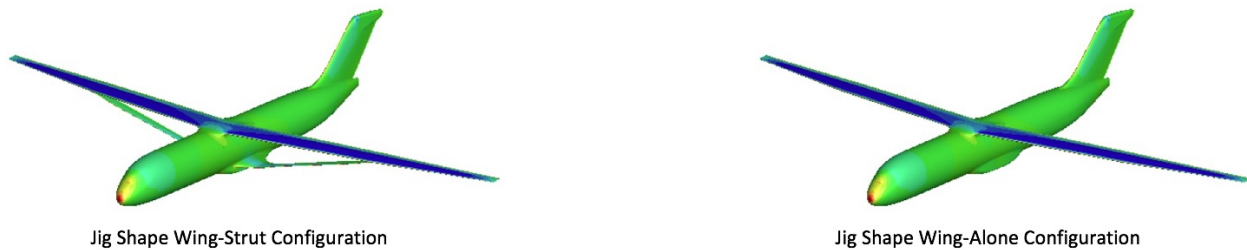
Figure 10. Jig Shape TTBW Wing-Strut Configuration and Wing-Alone Configuration in FUN3D
