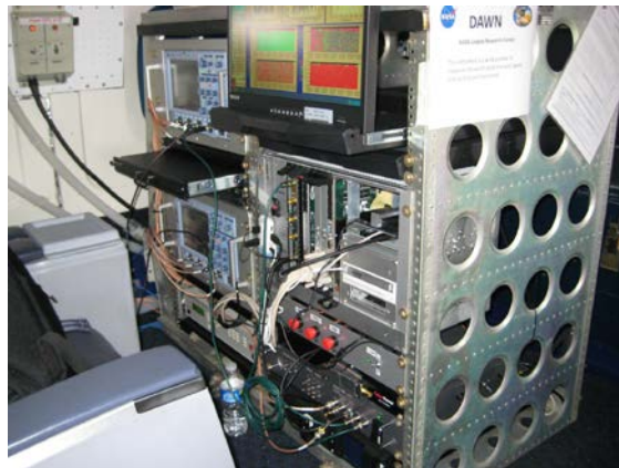
Figure 2. The picture of the DAWN airborne system showing the Lidar instrument control unit and the real-time data acquisition, processing, and display unit. Two operators control the system during airborne campaigns.
