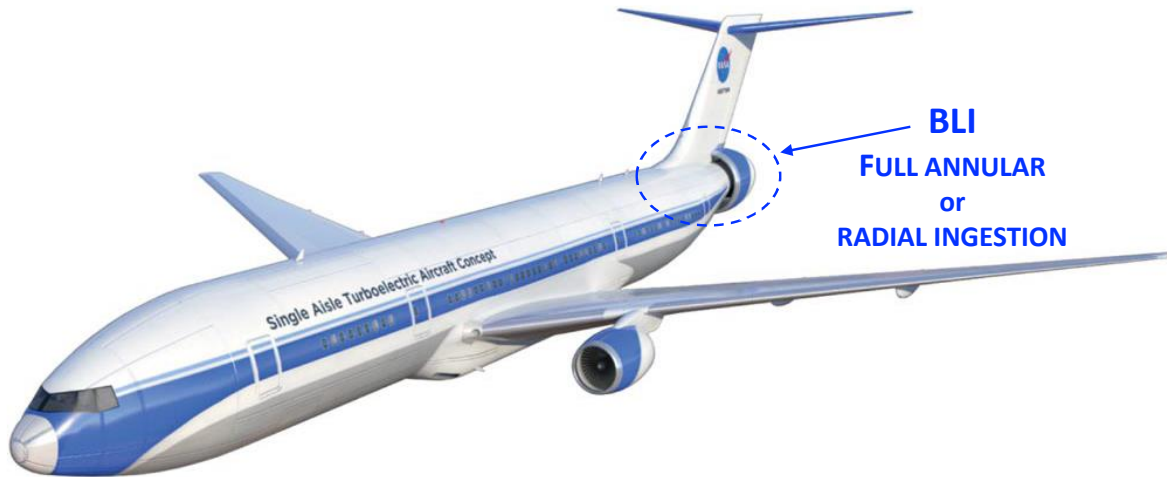
Figure 1. Tailcone propulsor concept with full annular BLI.
