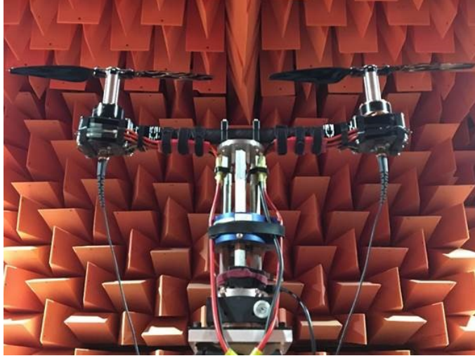
Figure 3 Testbed in the SALT facility.
