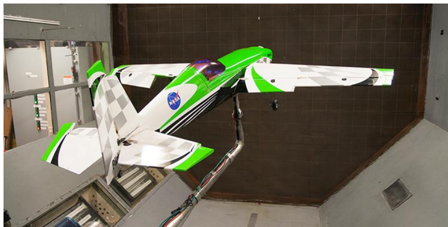
Figure 1. Conventional aircraft configuration (Mini-E) in LaRC 12-Foot Low Speed Tunnel.
