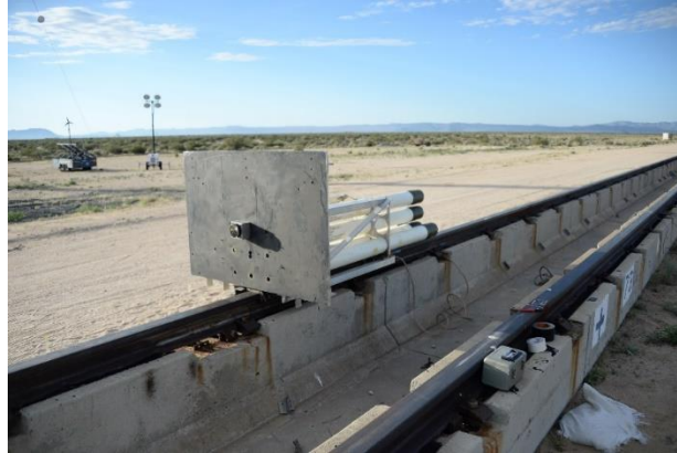
Fig. 1 Rocket sled with a diffuse target and a small retroreflector.
