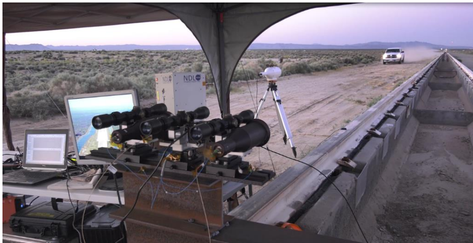
Fig. 2 NDL and its three transmit/receive telescopes placed on the end of the rocket-sled track.
