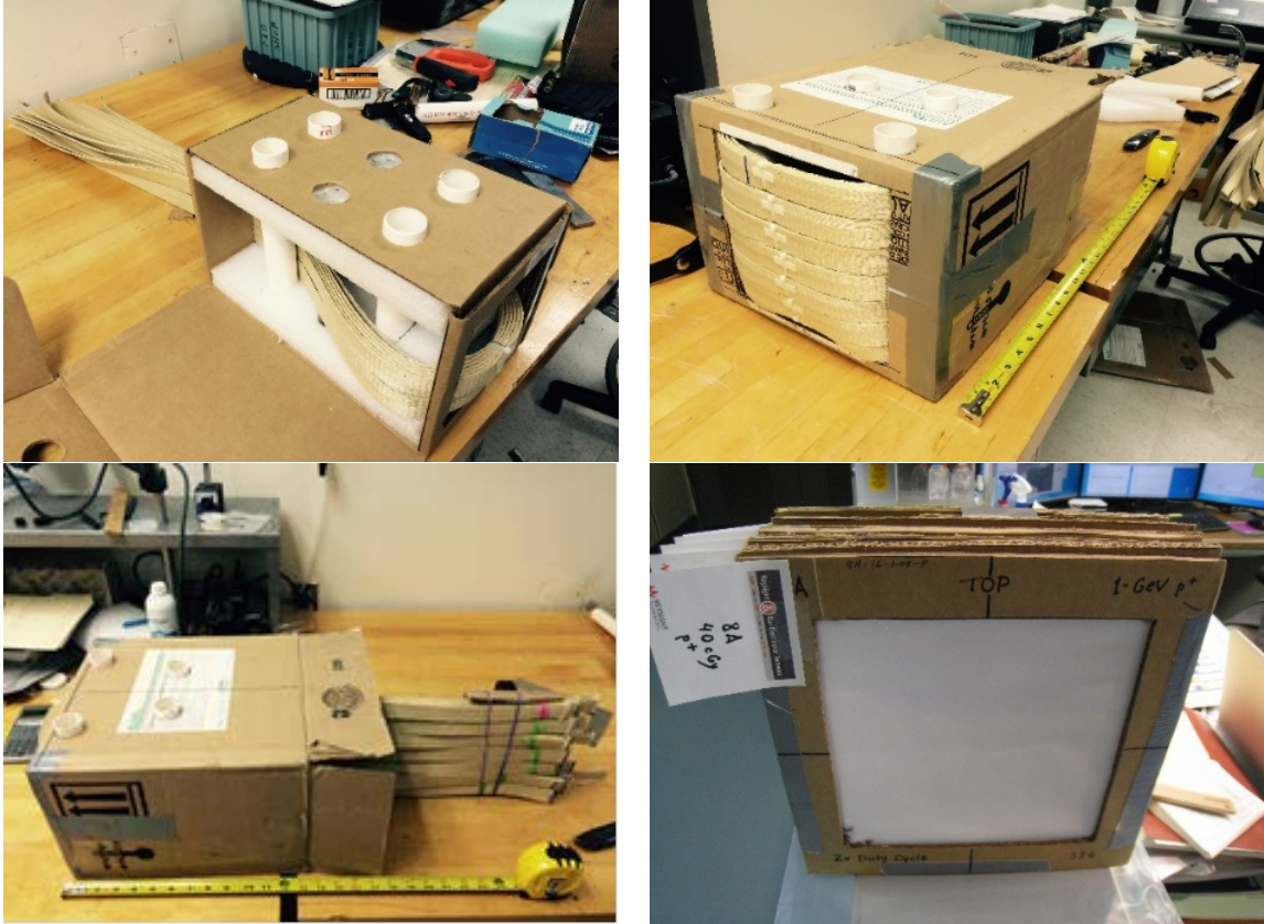
Figure 34 Representative fixturing with cardboard and low-Z materials.
