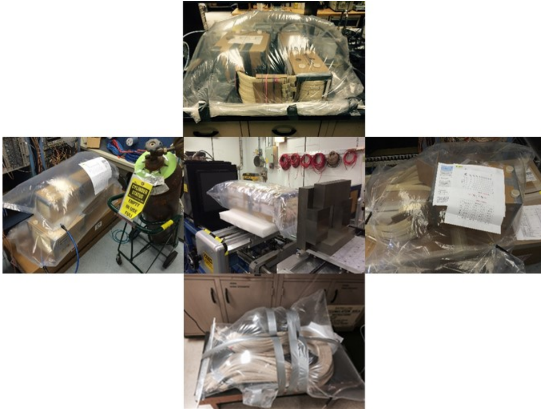
Figure 39 Conditioning of Vectran ® samples in argon before shipment to BNL (top), in argon before, during and immediately after irradiations at BNL (middle left, center, and right) and in nitrogen once samples were returned to WSTF (bottom).
