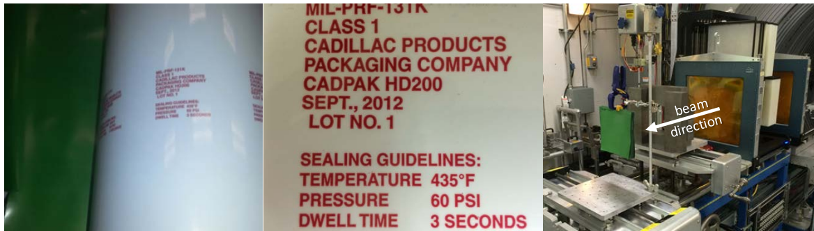
Figure 15 Cadpak® HD200 bladder material showing the original roll (left), space side writing (middle) and representative placement during the run 15-5A irradiation (right).
