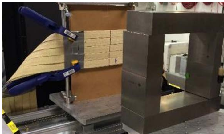
Figure 87 Run 15-13A schematic diagram for stacking sequence (5 layers high × 3 deep, left) and an actual picture of the 100-MeV iron Bragg peak run (right).
