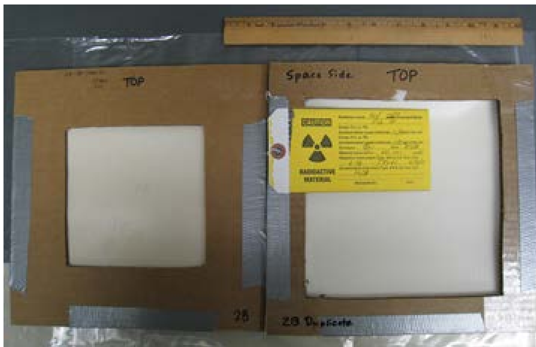
Figure 18 Fixtured Armorflex® ST10-5193-01 Lot A 15×15 cm (6×6 in.) stack (left) and Lot B 20×20 cm (8×8 in.) stack (right) (BNL NSRL Runs 16-2B and 16-2B DUP, respectively, space side).
