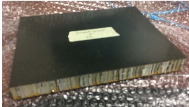
Figure 29 As-received sandwich core construction panel (20×20 cm, aluminum honeycomb core, filled with EX-1541 cyanate ester foam, inner mold line side facing up) (Run 17-3A).
