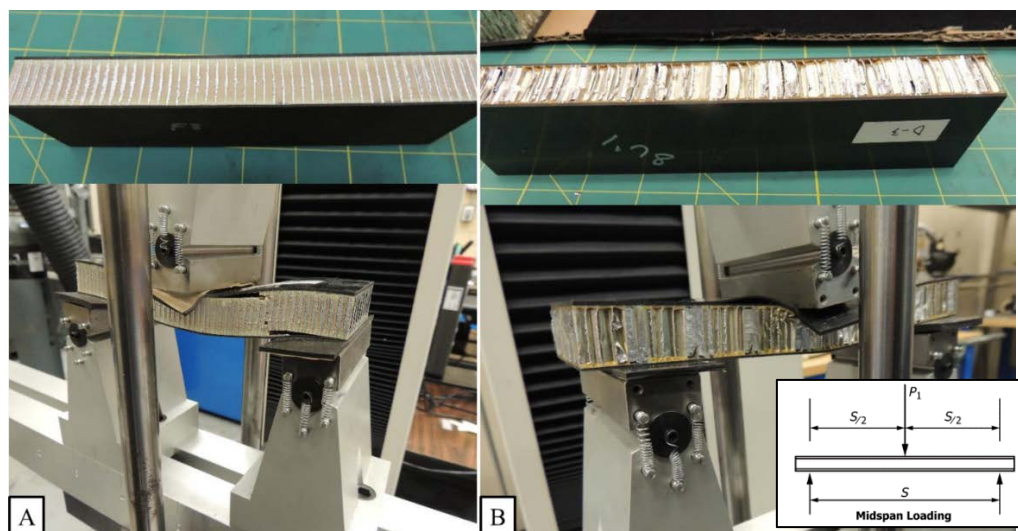
Figure 67 (A) Filled and (B) unfilled core test specimen prior to (top) and after failure (loading configuration shown in inset (lower right)).
