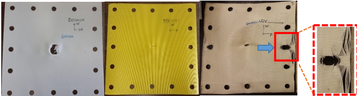
Figure 65 Puncture test specimens: Dacron® (left), polyurethane-coated nylon (center) and Vectran® (showing hole tearing) (right).
