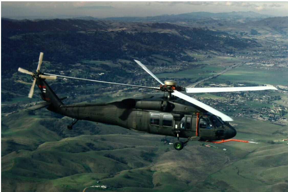
Figure 1. UH-60A with instrumented blades flying over the San Joaquin Valley during the UH-60A Airloads Flight Test Program.
