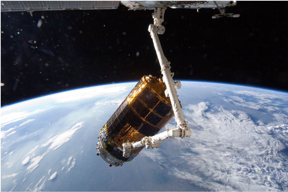
Figure 4. SSRMS capturing HTV before berthing. (Credit: NASA.)
