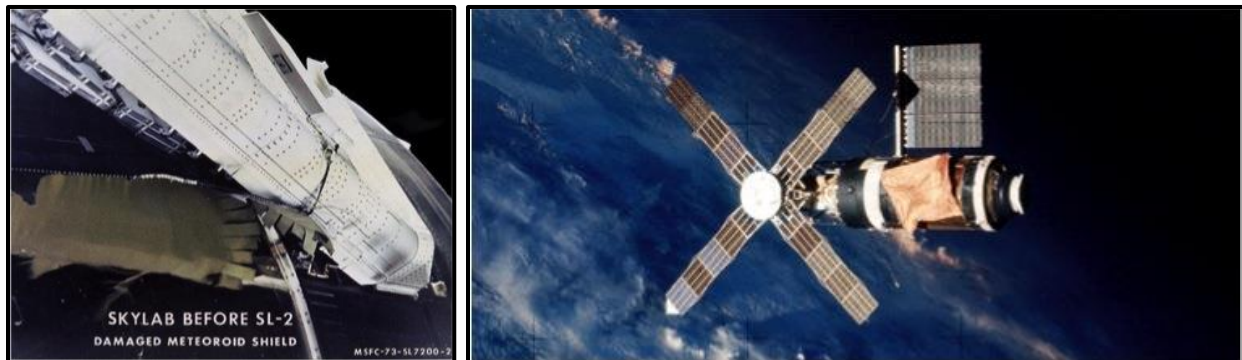
Figure 7.1-3. Skylab 1 Damaged Meteoroid Shield (left) and Solar Array Systems (right)
