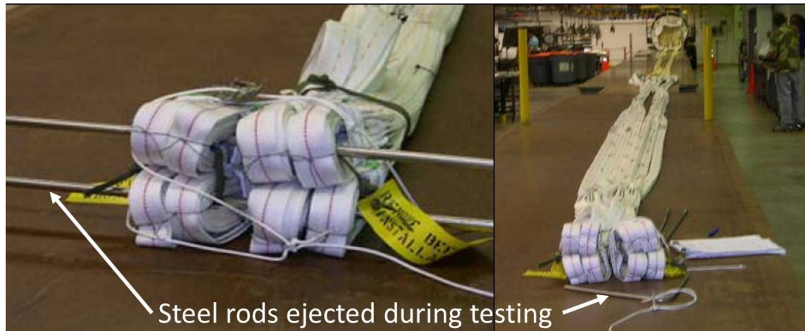
Figure 7.1-7. Parachute Riser Strip Test Setup
