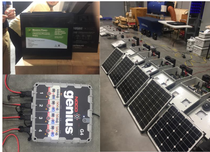
Figure 5-9 Lithium Iron Phosphate rechargeable battery (top left), trickle charger (bottom left), SBUDAS with solar panels prior to deployment at GAC Savannah GA (right)
