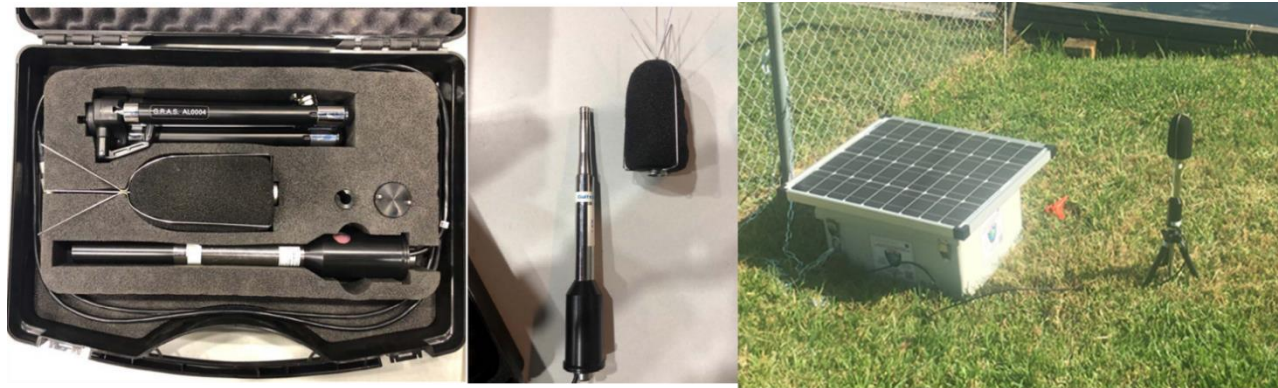
Figure 5-10 Left: GRAS Microphone with environmental enclosure and wind screen Right: SBUDAS with microphone mounted in environmental enclosure with wind screen on tripod as deployed during QSF18.
