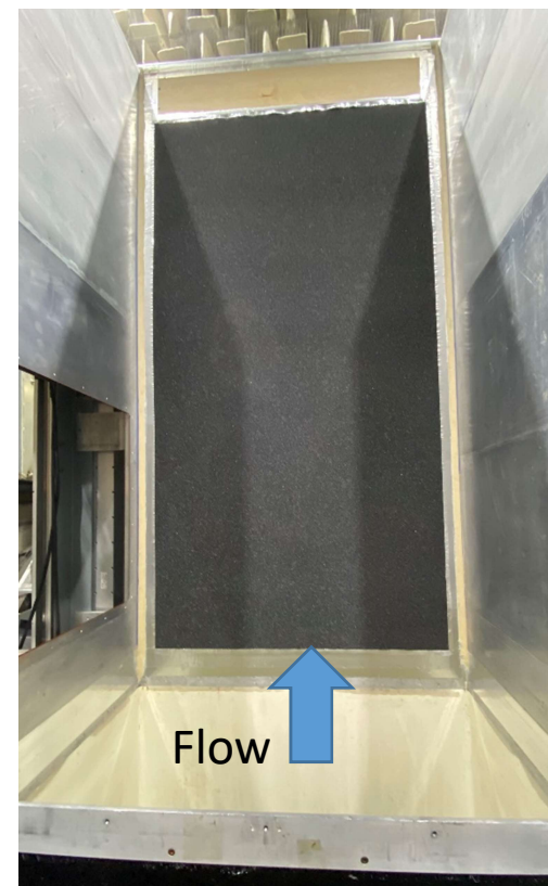
1" foam sheet glued to plywood panel
