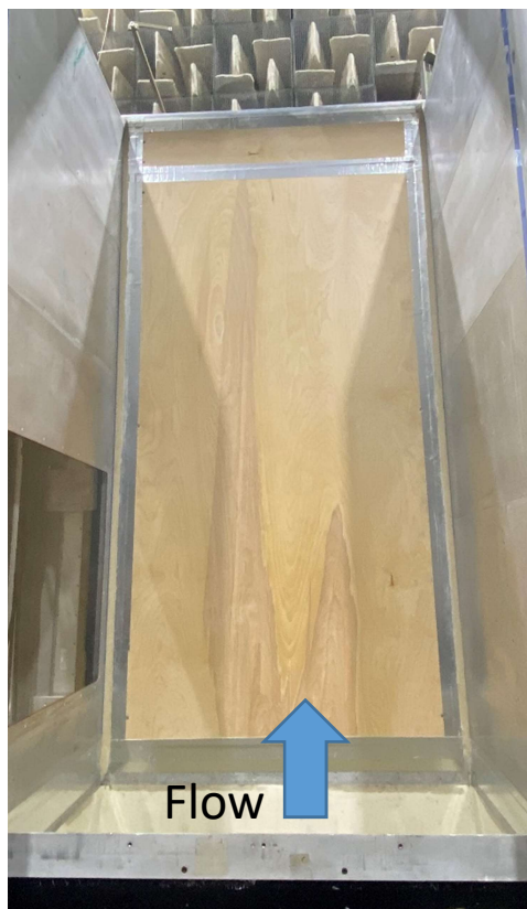
Plywood panel for "smooth surface" configuration
