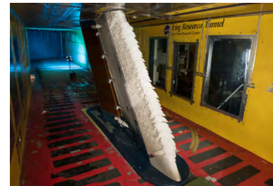
Ice Growth on 65% Scale CRM Wing Section Model
