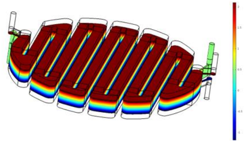
Figure 4. MFECR's model results: Potential (V) profile throughout GDEs and electrolyte
